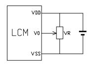
$V_{\text{DD}\sim}V_0\text{: LCD Driving voltage}$
